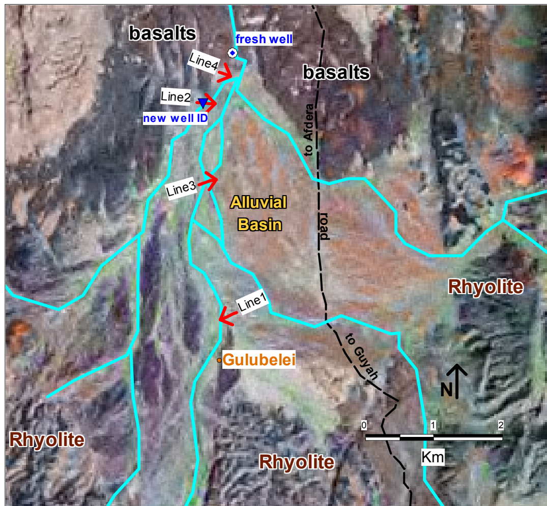
Fig. 10 Gulubele alluvial basin. Red arrows show length and direction of the geoelectrical surveys
